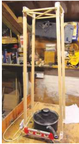
► Pic 2. Once he’d got the top and bottom shelves level, he used saucepans to work out the position of each intermediate shelf. Note, by the way, that the crossbars on the bottom shelf have broken out. He added panel pins later to reinforce the glue
